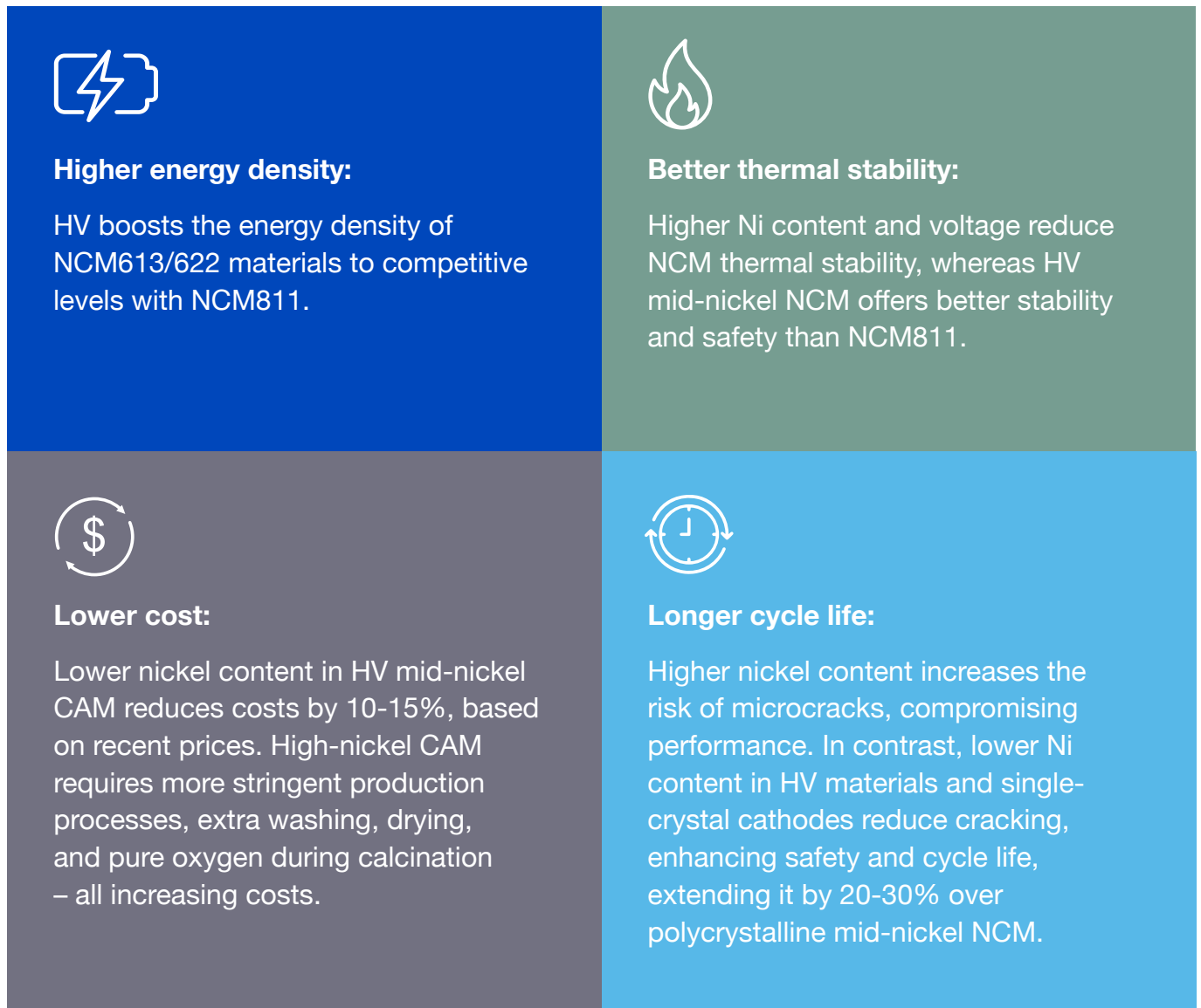
Figure 11: Benefits of high voltage (HV) mid-nickel over high-nickel
