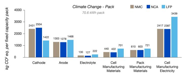
Lifetime emissions, including cradle-to-gate and use-phase emissions, for packs of a fixed 70.6 kWh capacity are broadly similar for all three chemistries. However, it should be noted that the climate change impact per battery for LFP is around 9% higher than NMC and NCA, when considering a 160,000 km use-phase in addition to battery manufacturing (Fig 3).
